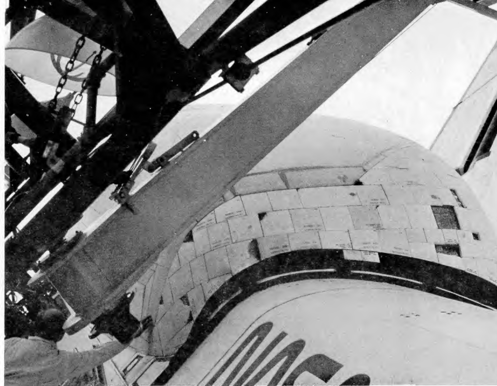
Figure 2-27.- Scorching of tile on forward edge of OMS pod.
