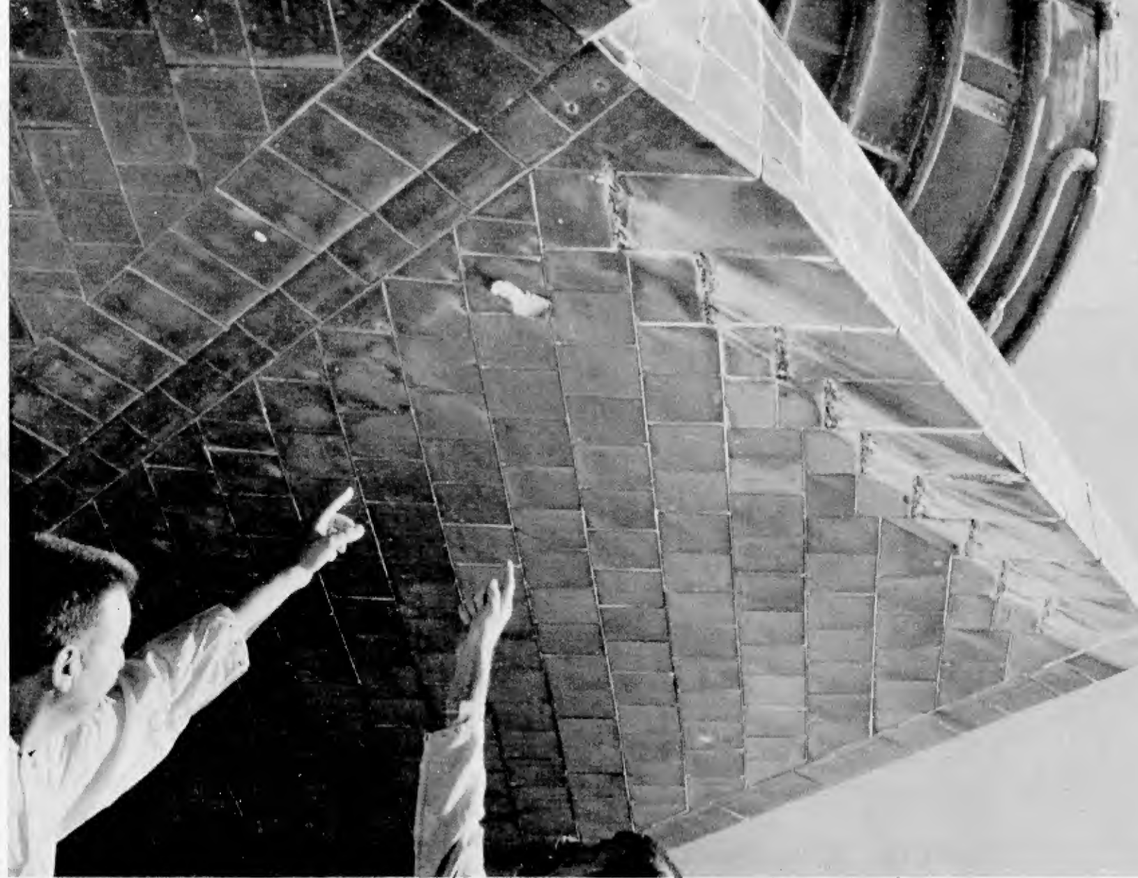
Figure 2-23.- Impact damage to left lower forward region of body flap.
